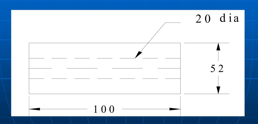
■ **Solution:** For determining processing time for components requiring more than one operation, always first determine the best possible sequence for manufacturing the component. To manufacture component shown in Figure 6.9, which requires three operations – facing, drilling and turning – any of the following sequences can be used
